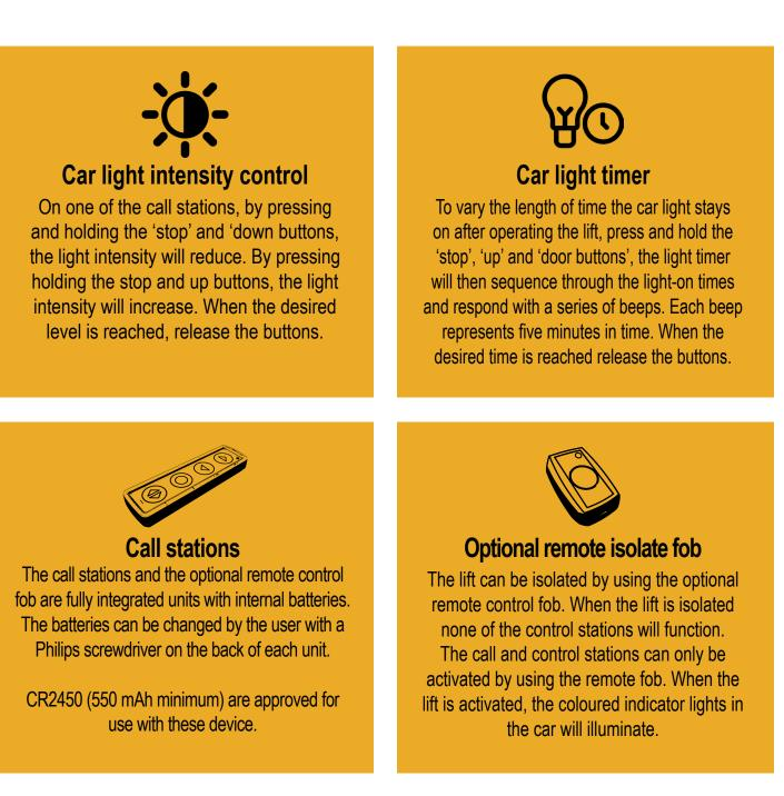
The lights in the car will switch on automatically when any call or control button is pressed and will automatically turn off after the pre-set time. (See 'Car light timer' above).
