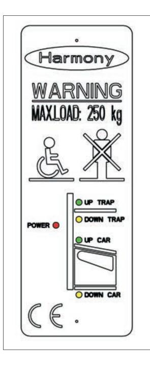
**UP TRAP** (green light) Infill panel safe edge OK. Will be off when descending.
