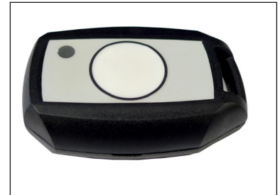
Remote enable fob The remote enable fob turns the lift on with a single press of the fob. The lift will stay on until a timer expires (default 6 min). Any subsequent presses of the fob with restart the timer. The remote mode and timer length can be set by an engineer on site to allow a user to get the functionality they require.
