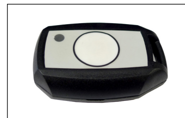
Remote enable fob turns the lift on with a single press of the fob. The lift will stay on until a timer expires (default 6 min). Any subsequent presses of the fob will restart the timer. The remote mode and timer length can be set by an engineer on site to allow a user to get the functionality they require.
