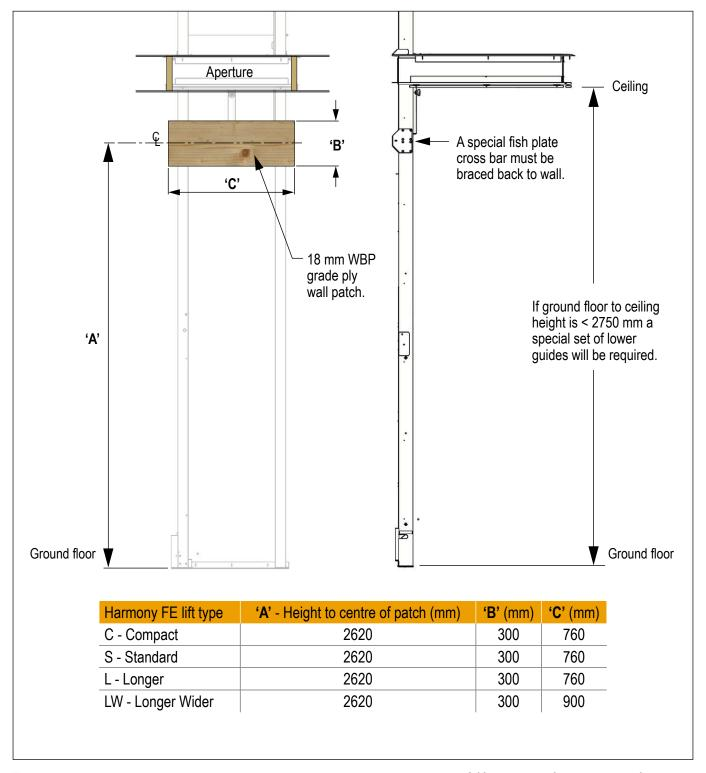
The lower guide brace kit can accommodate situations where the wall is up to 340 mm away from the rear of the aperture. If the distance is greater than this, a special bracing kit will be required.
