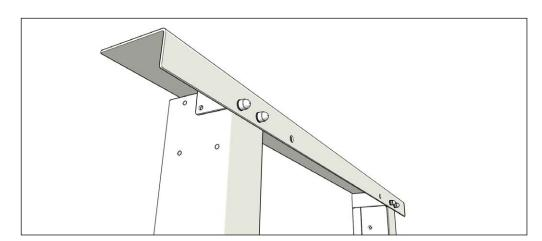
Fix Adjustable Ceiling Angle to cap.
