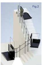
The compact and sturdy chassis is located 240 mm from the wall with the platform folded up and provides more space, particularly on narrow staircases. Landings can be safely passed using curves (Fig. 2) or by changing the inclination (Fig. 1). The rail is attached directly to the wall or to supports (Fig. 1 & 2). Multiple stopping points and parking positions can be individually planned.
